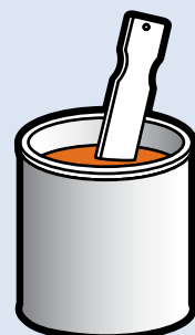
A Prepare color according to formula and reduce according to Technical Data Sheet. Use plastic or lined mixing container and only use plastic mixing sticks.
