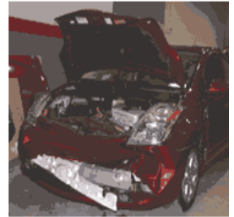
When a hybrid electric vehicle is mangled like this, there's always a chance that electrical components have been damaged, creating a potential hazard for the technician.
